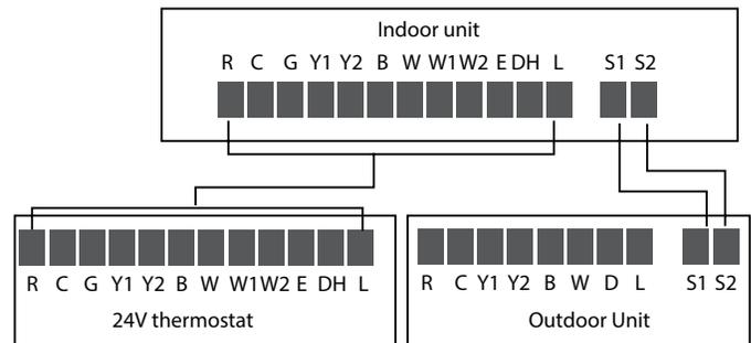
NOTE: The wiring method of the thermostat and the internal machine refers to the wiring of the non-communication scheme.
