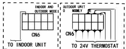
Outdoor unit wiring diagram:16022000036169
