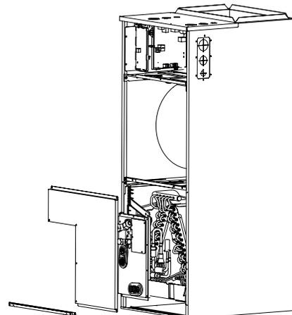
4. Unplug temperature sensors T1,T2,T2A,T2B and electronic expansion valve(EEV) from the control board.
