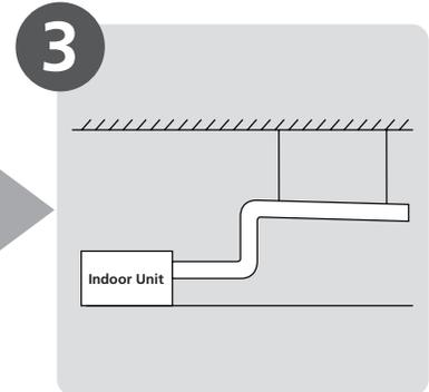
Install the drainpipe
