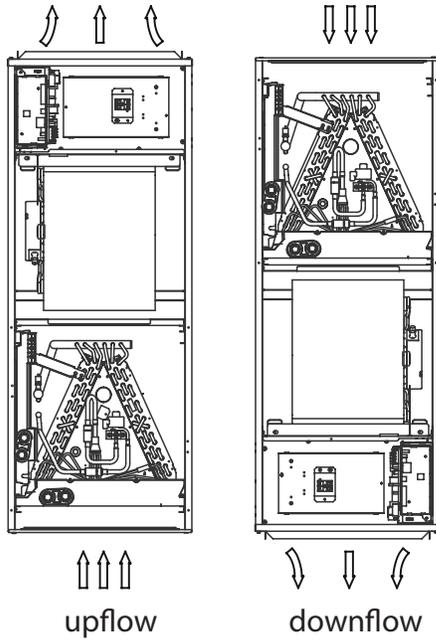
For the Horizontal left installation and vertical down installation, the direction of the evaporator should be changed and the drain pan should be removed first. Please do it according to the following steps:
