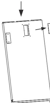
2. Remove the terminal block and power cord, loosen the screws, and remove the electric auxiliary heating cover.
