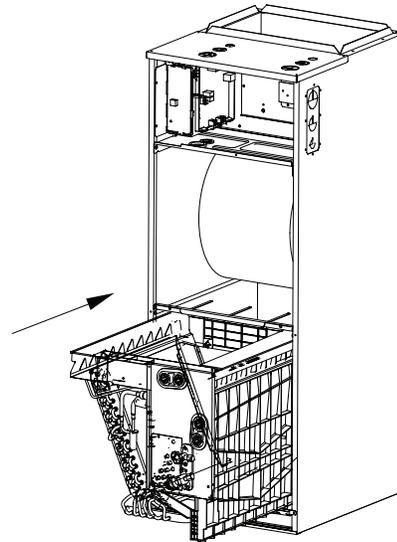
8. Reinstall T1,T2,T2A,T2B sensor plug and electronic expansion valve(EEV) and tie up the sensor wires.
