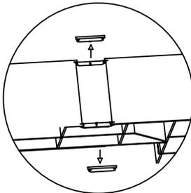
Remove knockouts as shown in the figure.
