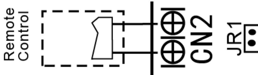
B. For remote control (ON-OFF) terminal port CN2 and short connector of JR1
