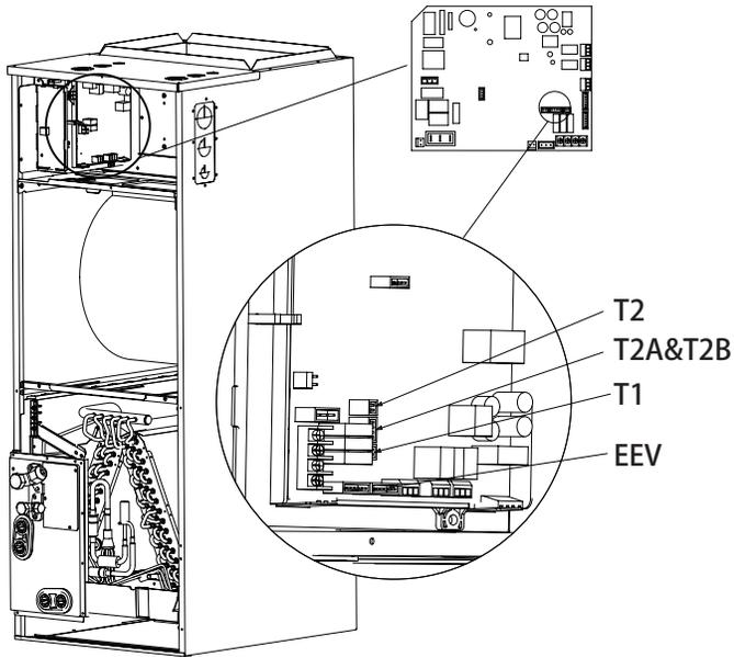
5. Remove T1,T2,T2A,T2B sensor,EEV wire ties.
