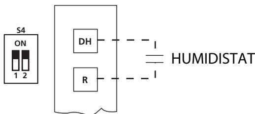
Dehumidification control requires indirect humidifier at DH and R. Set S4-2 as OFF. When the humidity rises and exceeds the set value of the humidifier, the 24V
