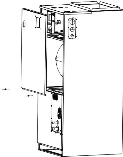
14. Reinstal the filter and filter cover plate.
