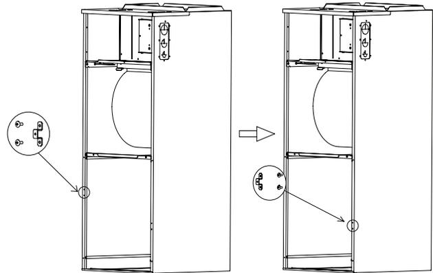
8. Reinstall the evaporator and drain pan.
