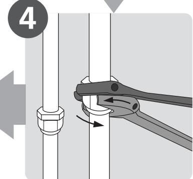
Connect the refrigerant pipes
